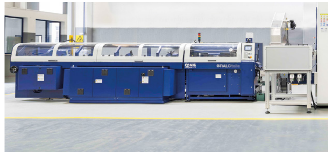
Segatrice, tramoggia e tazza vibrante Sawing machine, hopper and vibrating bowl feeder
