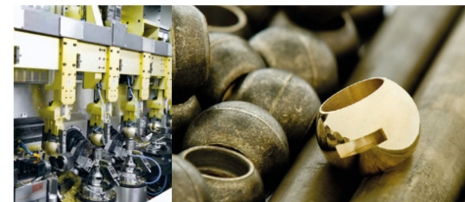
Sfera con forature trasversali multiple. Ball with multiple cross drilling.
